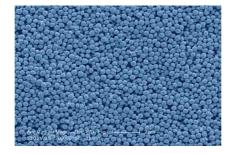
A solvothermal route for the size-controlled synthesis of ferromagnetic submicrometer  $Fe_3O_4$  spheres is described. The formation of small nanoparticles and their subsequent oriented assembly lead to microspheres with a remarkable "single-crystalline" feature. The spherical  $Fe_3O_4$  aggregates could serve as substrates to grow  $Fe_3O_4$  nanorods, which provides an alternative method for the preparation of  $Fe_3O_4$  1D nanostructures.
